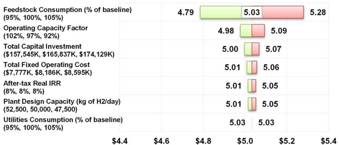
FIG. 14. Tornado chart of cost distribution of hydrogen produced using a PEM electrolyser.
